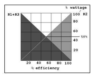
The majority of the impedance, of the feed point resistance, will be due to R3 or the ground resistance, and the inductive reactance of the extra large coil portion. The feed point impedance will be mostly defined as R3 jX +XL
