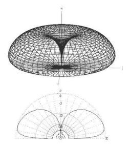
This software graphical snap shot is believed to be the far field pattern; as best as the softwares can interpret the short 3 meter height antennas herein. And this is an actual model of such 3 meter antennas. Not just a .....
