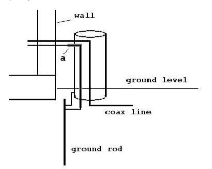
This Farady Cage cylinder is partly in the ground. The ground wire going into the cage at a. is insulated so it does not short to the cage. The cage should be located very close to the building wall.
