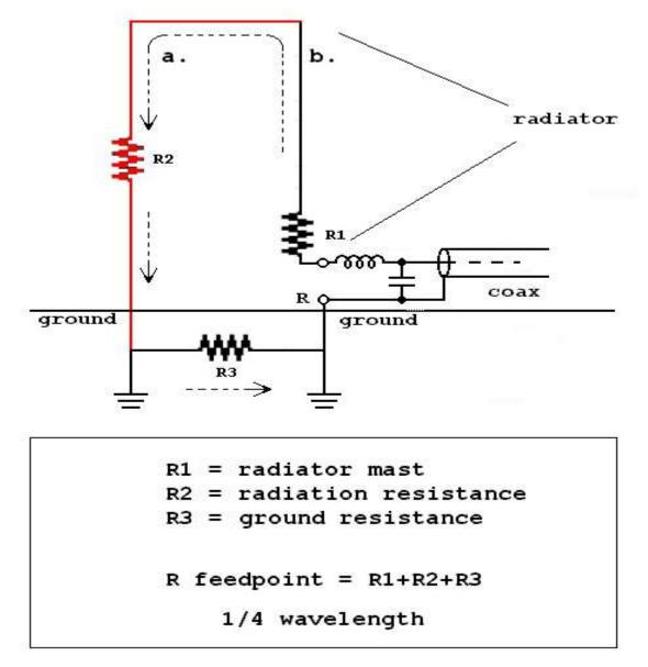
This is the typical equivalent circuit of an antenna. And R1 = the ohmic resistance of the radiator plus it's coil ohmic resistance if there is a coil in the radiator section. Not to be confused with the a coil's reactance jX (+XL). R2 = the radiation resistance. R3 = the ground resistance. The radiation resistance is high in the case of a  $\frac{1}{4}$  wavelength radiator. As compared to the short height antenna of less height than the  $\frac{1}{4}$  wavelength.
